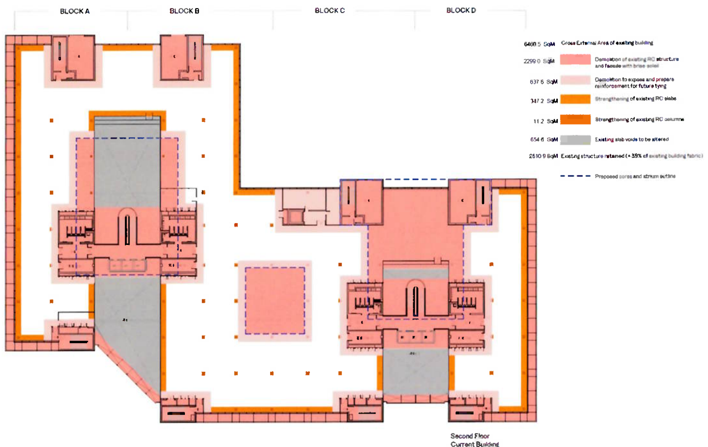
Figure 1 Demolition plan in the R&E option
